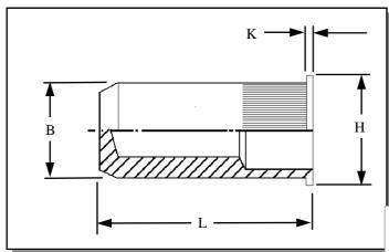
Round flat head closed ended Knurled body Rivetnuts for material up to 5.50 mm thick.
