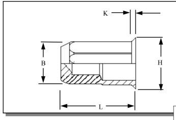
All Hexagon low profile head closed end Rivetnuts for material up to 3.00 mm thick
